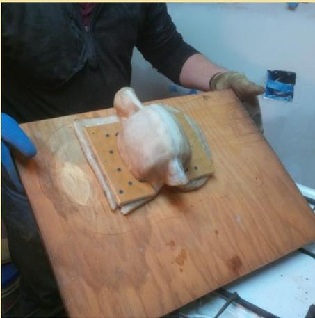
Finished elbow mold using clamps, ready to go back in the oven. I use less excess plastic now.
