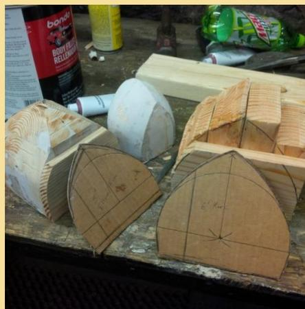
Making elbow molds from wooden blocks and finishing with bondo.
