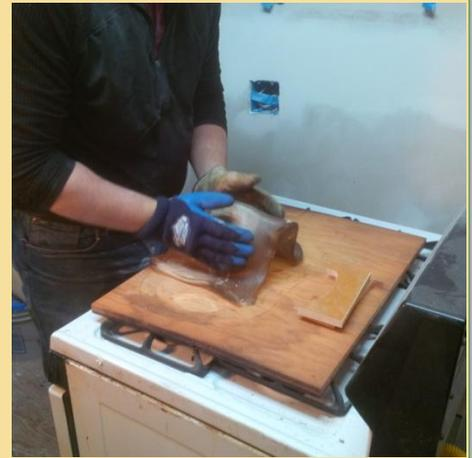
Molding hot plastic onto an elbow form.
