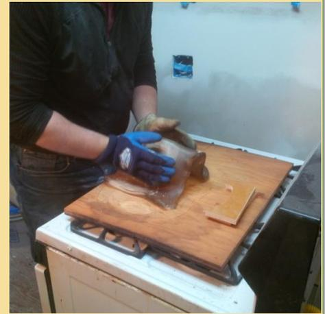
Molding hot plastic onto an elbow form.
