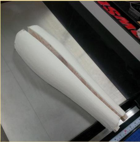
Front half of greave mold. Hardware cloth covered in plaster. Made in two parts to allow for different sized legs, adjust with wedges.
